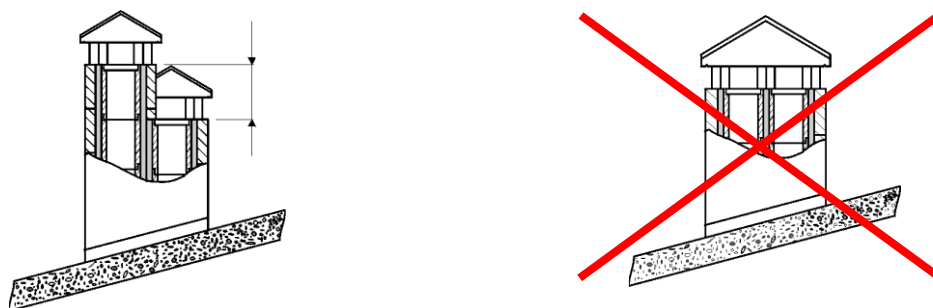
Figure 8. Construction of adjacent chimneys.
