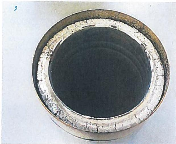
*Photo 4: Chimney element 1 after thermal tests*
