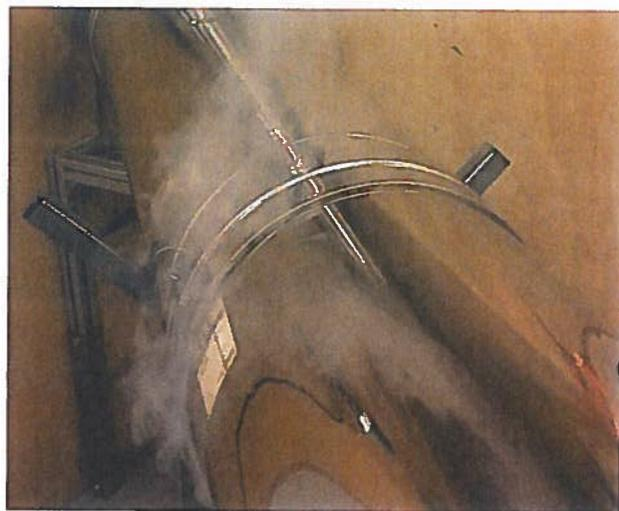
*Photo 5: Smoke from joint during heat shock test*
